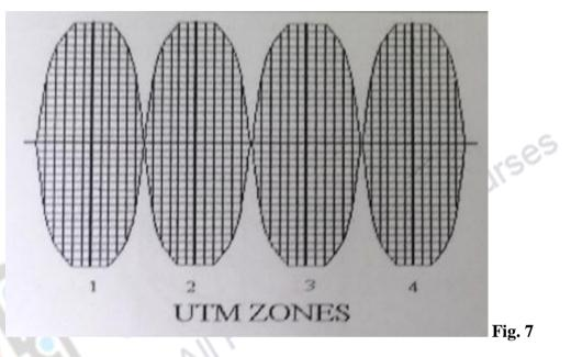
The central meridian is a great circle and is the only line represented by a straight line in the map projection. Each UTM zone divided into vertical bands of 8 latitudes. These bands are identified by letters, south to north; starting with 80° south with letter C and ending with letter X. Letter I and O are omitted whereas letter A, B, Y, Z are reserved for Universal Polar Stereographic Coordinate System. Each UTM zone is in fact a different projection using a different coordinate system.
